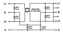
Match the corresponding L1 & L2 terminal lugs for the input and output phase wires when connecting a split phase configuration.
