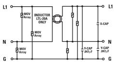
Use only the L1 Terminal lug for the phase wires (input & output) when connecting LoadTrack LTL in a single phase configuration.
